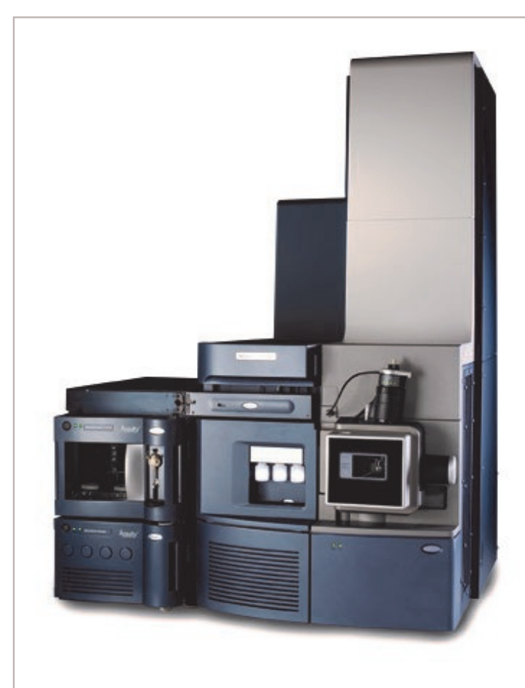
Figure 2. ACQUITY UPLC system coupled to Xevo G2 QToF
